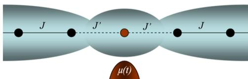
Fig. 1 Schematic setup of a one-dimensional chain with a periodically driven impurity, modelled by an oscillating chemical potential. The blue shaded areas indicate the regions of the leads and the impurity.
