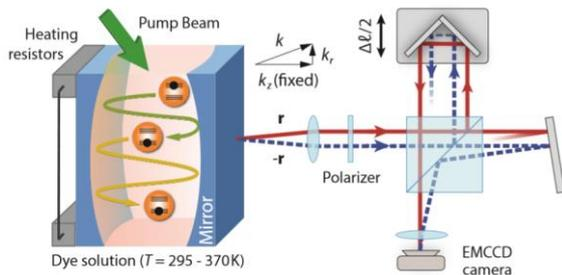
Fig. 3 Dye filled microcavity confining a two-dimensional gas of photons with effective mass. To investigate the transversal and longitudinal coherence a Michelson interferometer is used.
