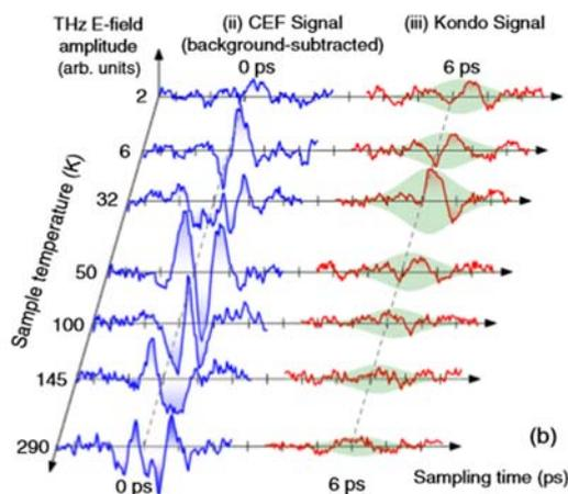
**Figure 3:** Evolution of the background-subtracted signal ( $-2.5$  to  $+2.5$  ps) and the Kondo signal ( $+3.5$  to  $+8.5$  ps) as the temperature decreases from 290 to 2 K.
