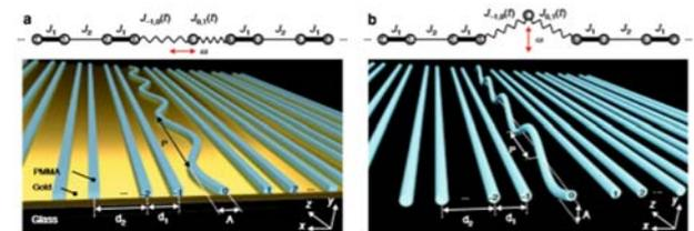
**Figure 4:** Sketches of the SSH chains with time-periodic perturbations of a single lattice site at the interface between two distinct dimerisations (top) and the corresponding experimental realisations (bottom).
