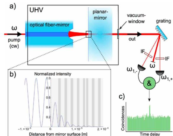
Fig. 1 (a) Scheme of the setup. (b) Calculated intensity distribution in the optical coating of the mirror. (c) Measured pair correlations.
