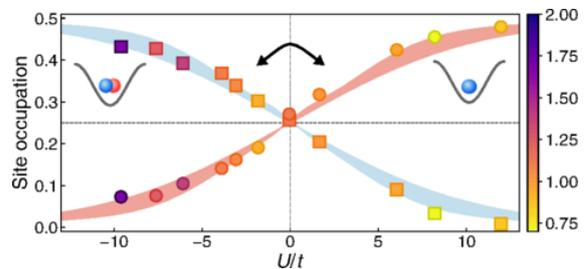
Fig. 2: When reversing the sign of the interaction  $U$  singly occupied sites (circles) with spin-up should be mapped to doubly occupied sites (squares). Particle-hole symmetry correspondingly here reflects in the mirror symmetry around the vertical line at  $U=0$ .
