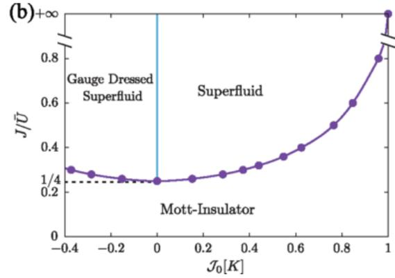
Fig. 4: Phase diagram of the kicked system. For strong kicks, corresponding to  $J_0[K] < 0$ , a novel superfluid phase emerges.
