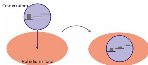
Fig. 1: A cesium atom is placed into a rubidium cloud, and by thermal contact the spin states equilibrate. For simplicity only 3 spin states are shown.
